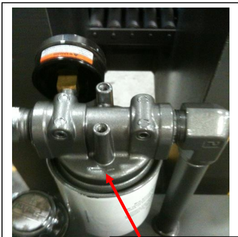
Notice direction of arrow on filter assembly housing pointing back to the return to tank line.
